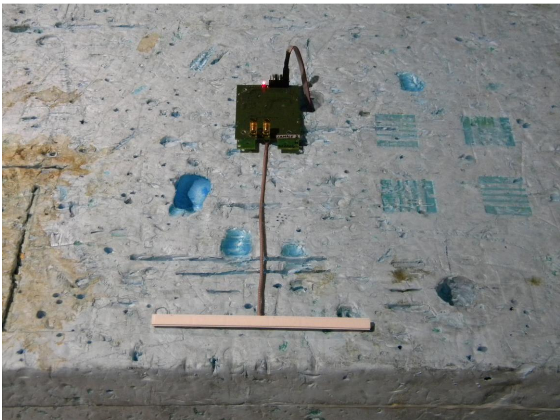
Photograph 2. Radiated emissions test setup, antenna 2.
