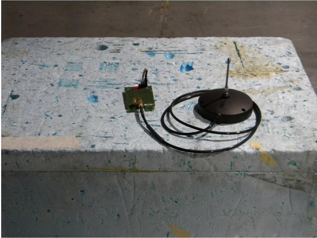
Photograph 3. Radiated emissions test setup, antenna 3.
