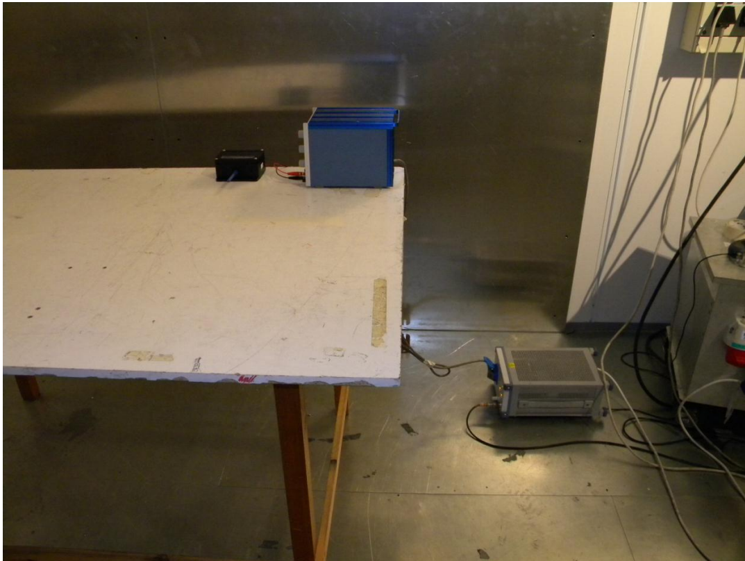
Photograph 3: AC power line conducted emissions test setup, EUT 1
