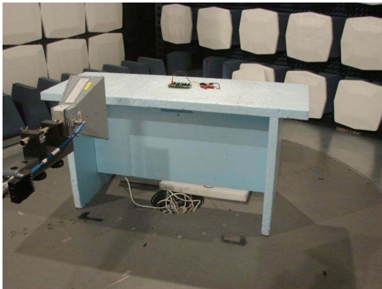
Picture 2: Receiver Radiated emission test setup 1 GHz – 10 GHz
