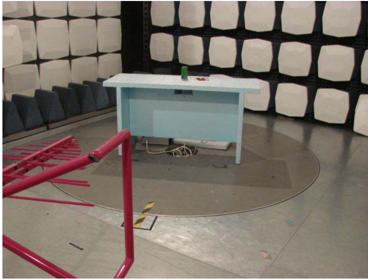
Picture 1: Receiver Radiated emission test setup <1 GHz
