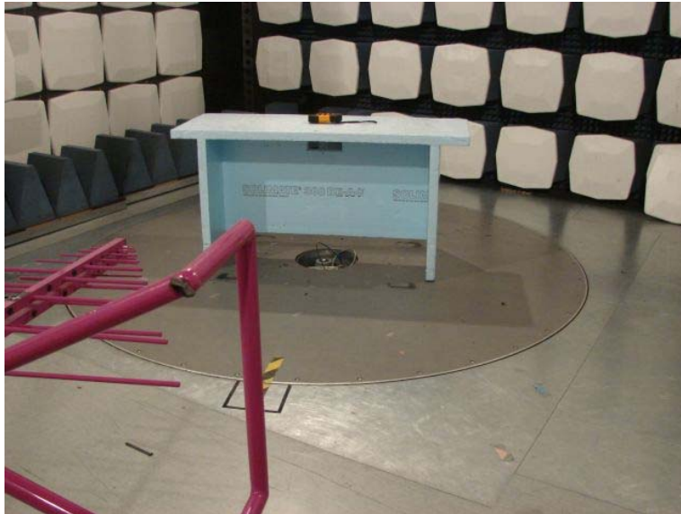
Picture 5: Transmitter Radiated emission test setup <1 GHz
