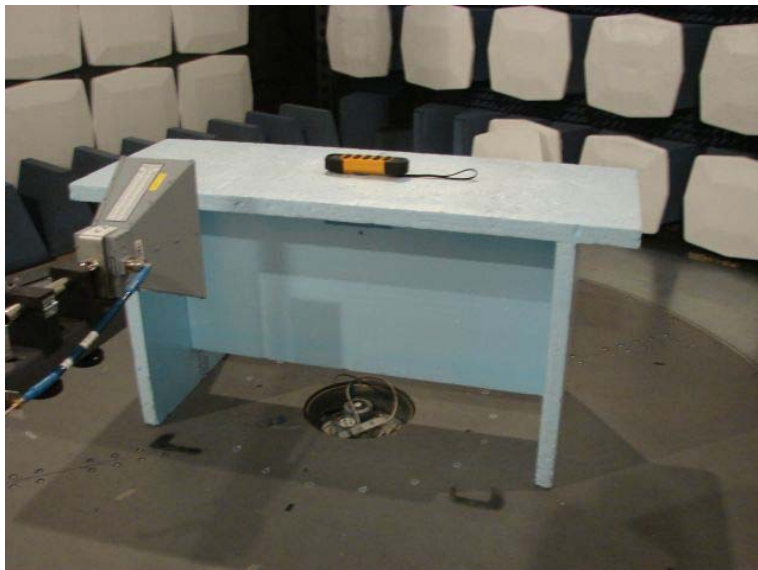
Picture 6: Transmitter Radiated emission test setup 1 GHz – 10 GHz.
