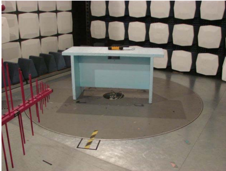
Picture 5: Transmitter Radiated emission test setup <1 GHz
