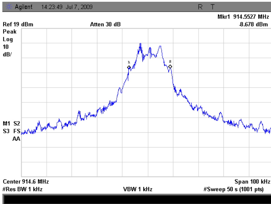
Picture 28: 99% Bandwidth measurement result; middle channel
