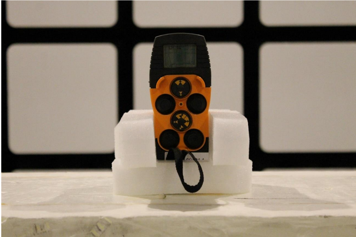
Photograph 11. EUT position during radiated tests
