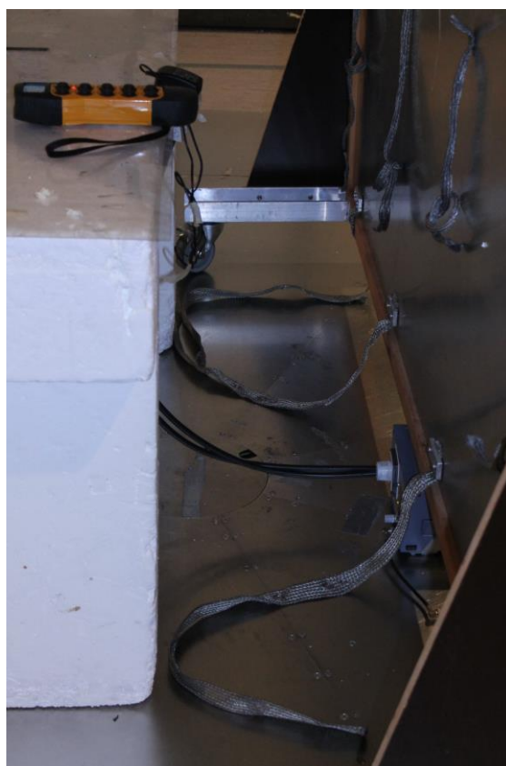
Photograph 2. Conducted emissions at mains ports 0.150 – 30 MHz
