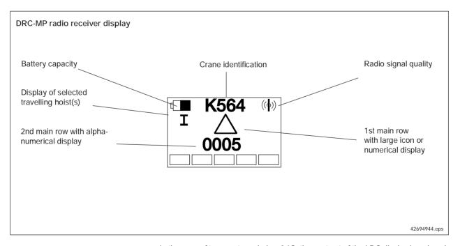
In the case of temperatures below 0  $^{\circ}$ C, the contrast of the LDC display is reduced and the time for changing the characters increases.
