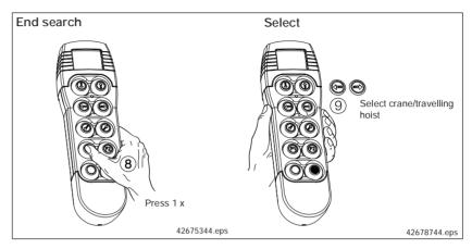
After starting selection with F1, the crane identification of the controllable radio receivers can be displayed one by one by scrolling with the Left and Right keys
