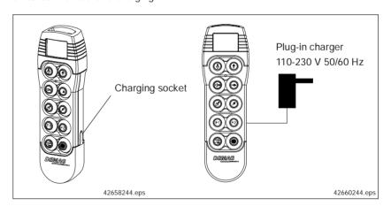
The charging process is monitored and controlled by the electronics in the handheld transmitter. Partly discharged batteries can also be charged.
