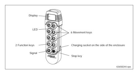
The LED in the hand-held transmitter indicates the operating status of the hand-held transmitter:
