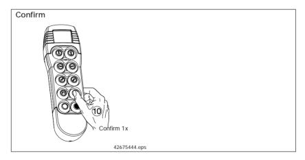
By pressing the F2 key for confirmation, the hand-held transmitter is assigned to the DRC-MP or DRC-DR radio receiver whose crane identification is shown in the second main row of the display (NOID in the example). At the same time, the crane identification of the DRC-10 hand-held transmitter is also changed to the new value and displayed next to the battery icon.
