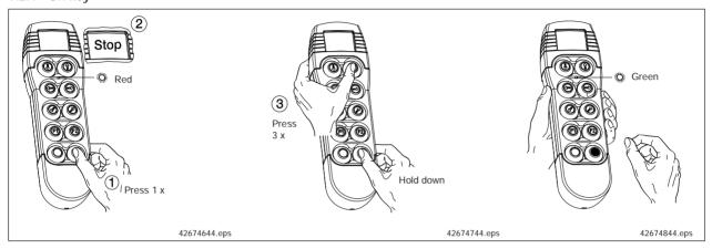
The LED in the display field flashes green if Run mode is switched on after entry.
