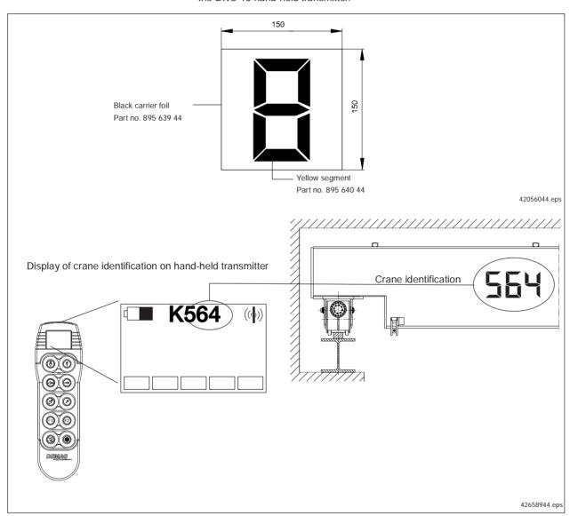
The coding labels (dimensions  $150 \times 150 \text{ mm}$ ) (black background foil + foil with number) must be fitted on the hoist unit in such a manner that they are easily visible.
