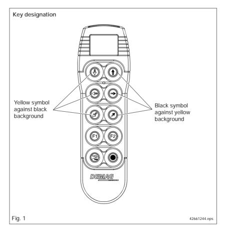
As standard, all keys on the hand-held transmitter are designated in the factory with the relevant foil symbols.
