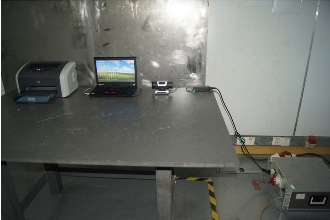
Photograph 6: Set-up for Radiated Emissions, below 1GHz
