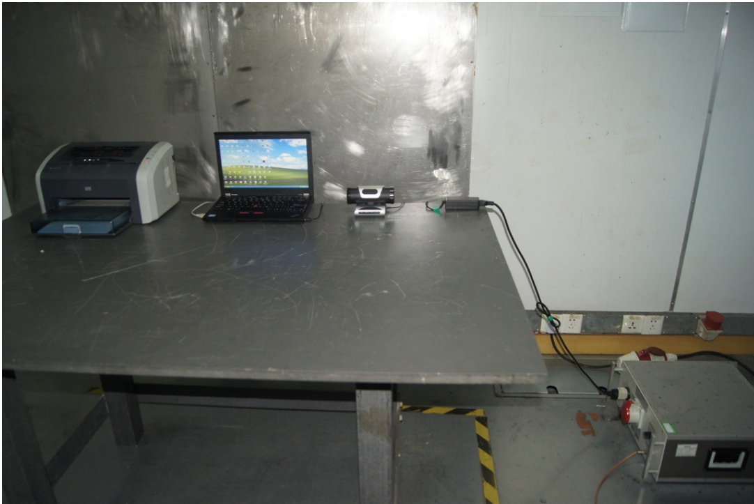
Photograph 6: Set-up for Radiated Emissions, below 1GHz
