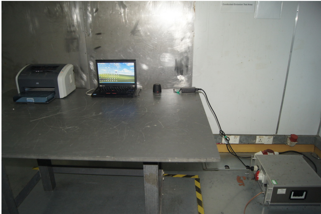
Photograph 6: Set-up for Radiated Emissions, below 1GHz
