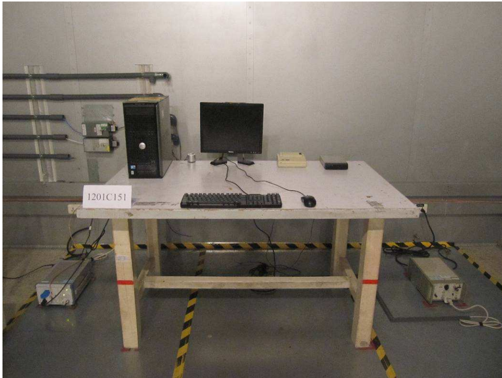
Photograph 4: Set-up for Spurious Emissions, below 30MHz
