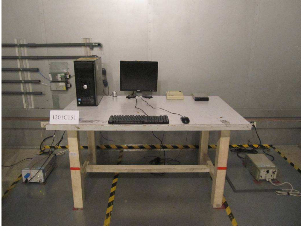
Photograph 4: Set-up for Spurious Emissions, below 30MHz
