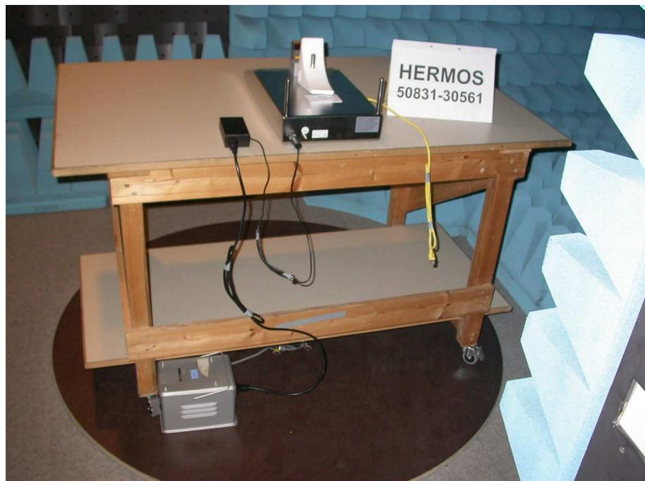
**Test setup for radiated emission measurement
