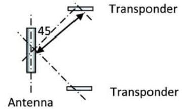
Perpendicular (frame antenna) The illustration shows the optimal position of the transponder if it is perpendicular to the axis of a frame antenna.
