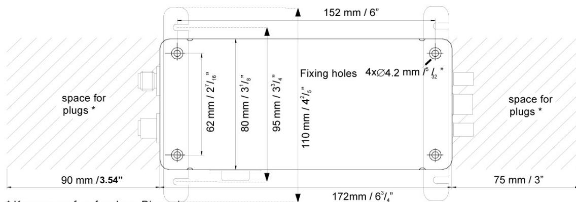
\* Keep space free for plugs. Dimensions for straight cable plugs. Angled cable plugs decrease space.
