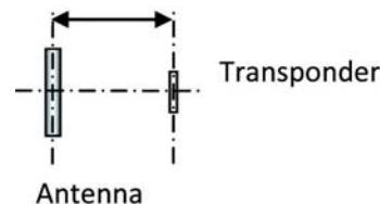
Perpendicular The illustration shows the optimal position of the transponder if it is perpendicular to the axis of the antenna.
