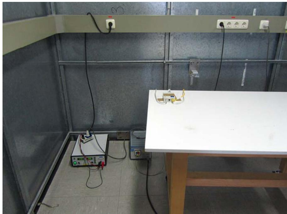
**Test setup for conducted DC powerline emission measurement**
