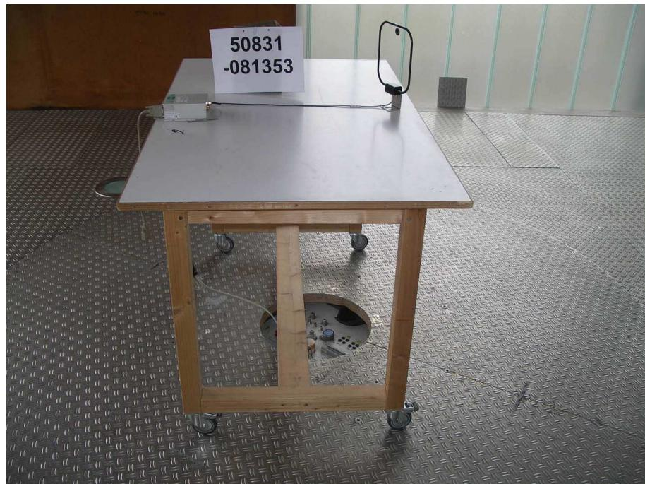
**Test setup for radiated emission measurement
