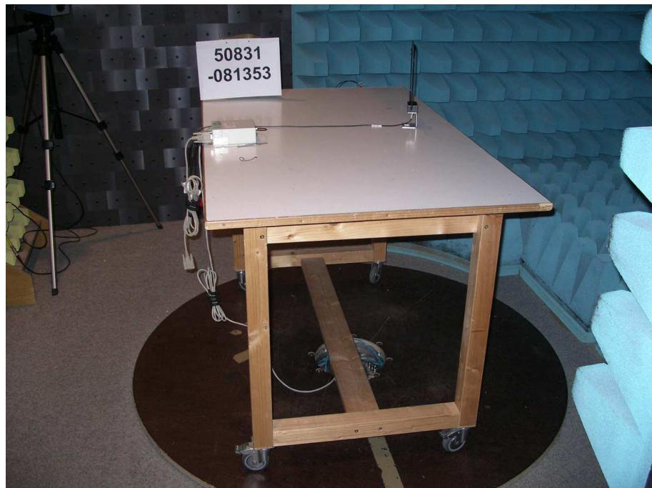
**Test setup for radiated emission measurement
