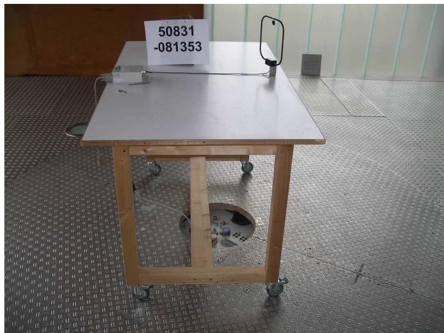
**Test setup for radiated emission measurement
