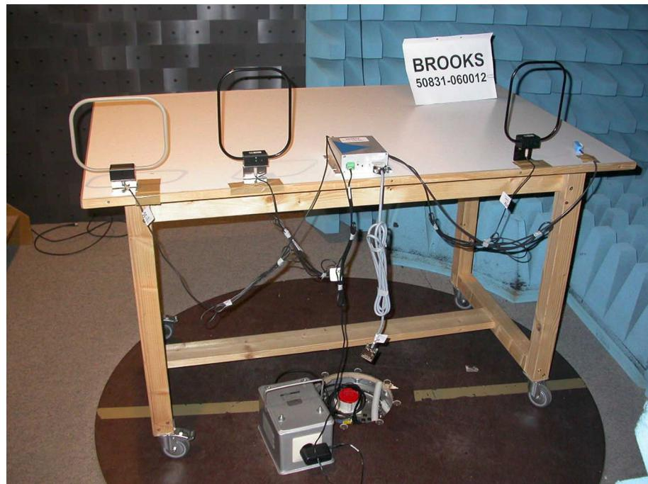
**Test setup for radiated emission measurement
