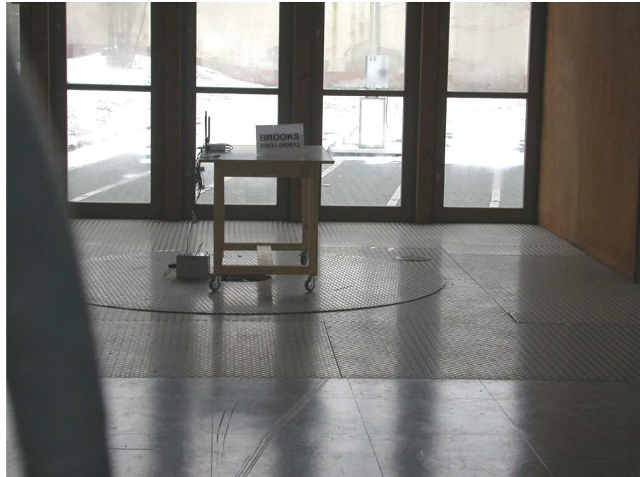
**Test setup for radiated emission measurement
