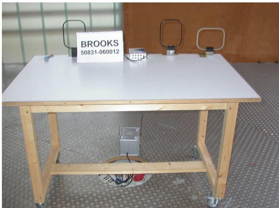
**Test setup for radiated emission measurement
