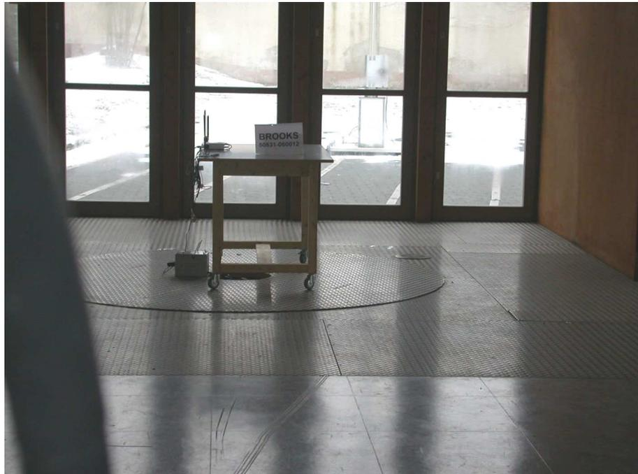
**Test setup for radiated emission measurement
