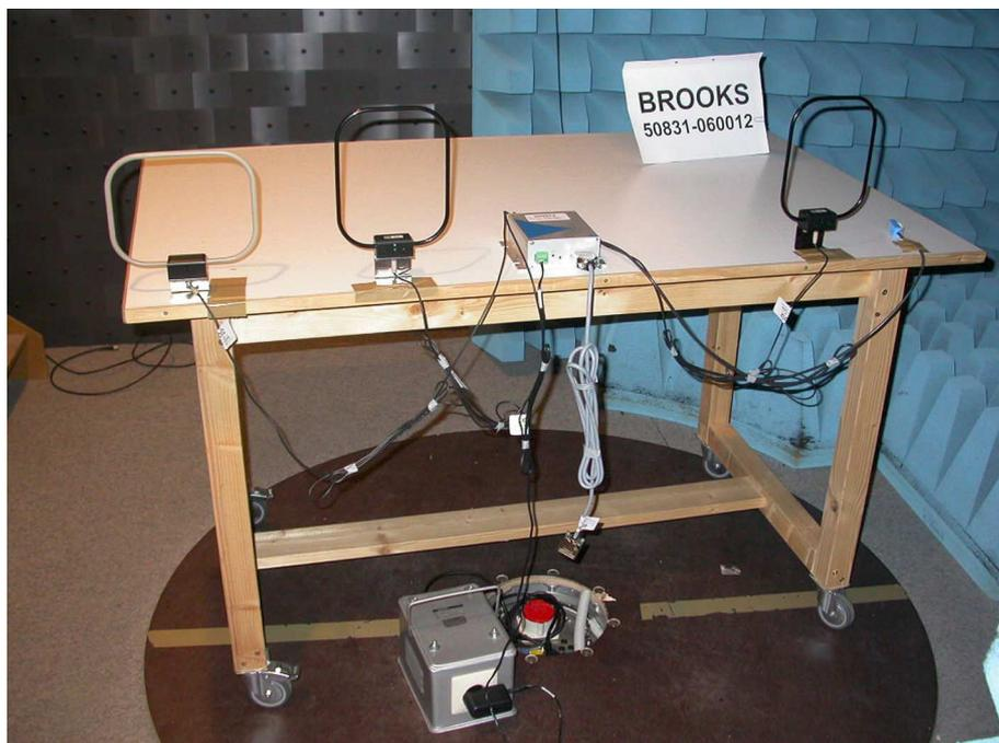
**Test setup for radiated emission measurement
