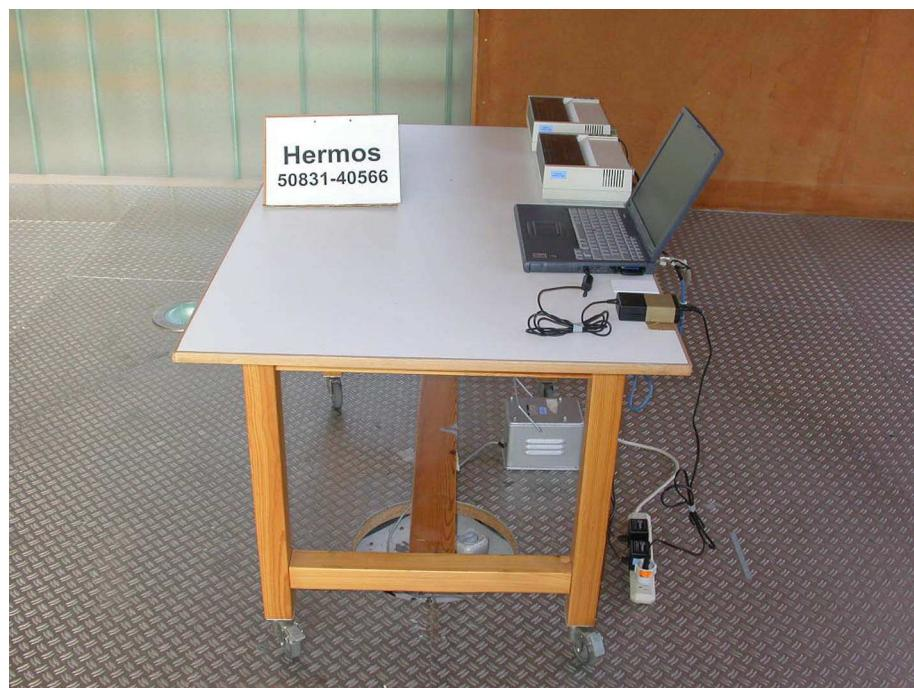
**Test setup for radiated emission test
