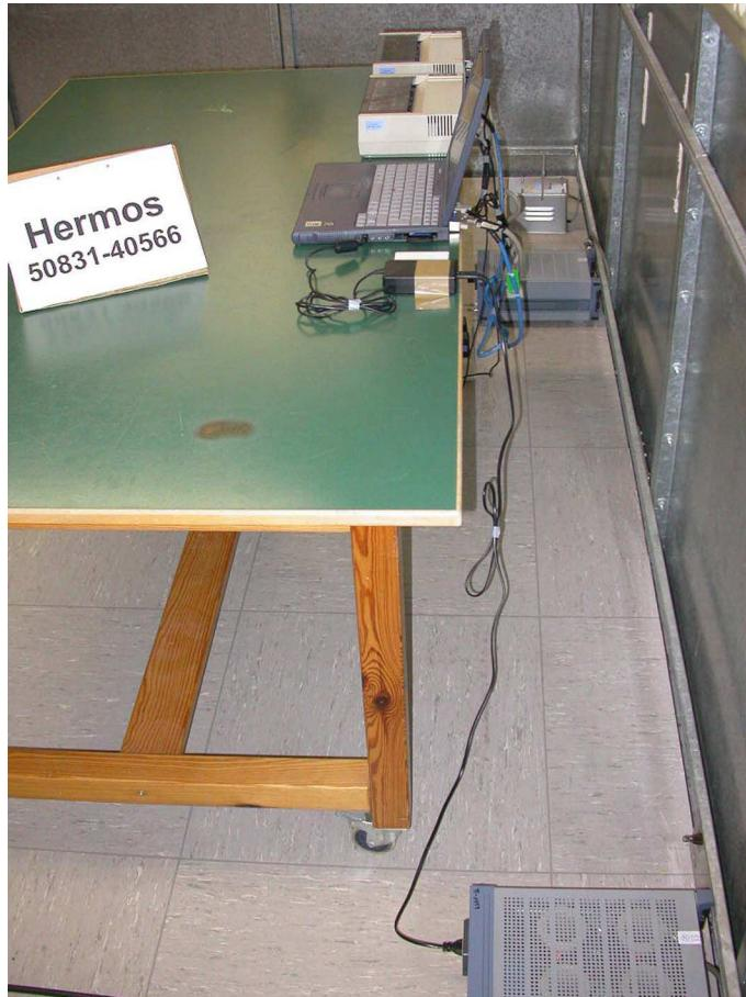
**Test setup for radiated emission test
