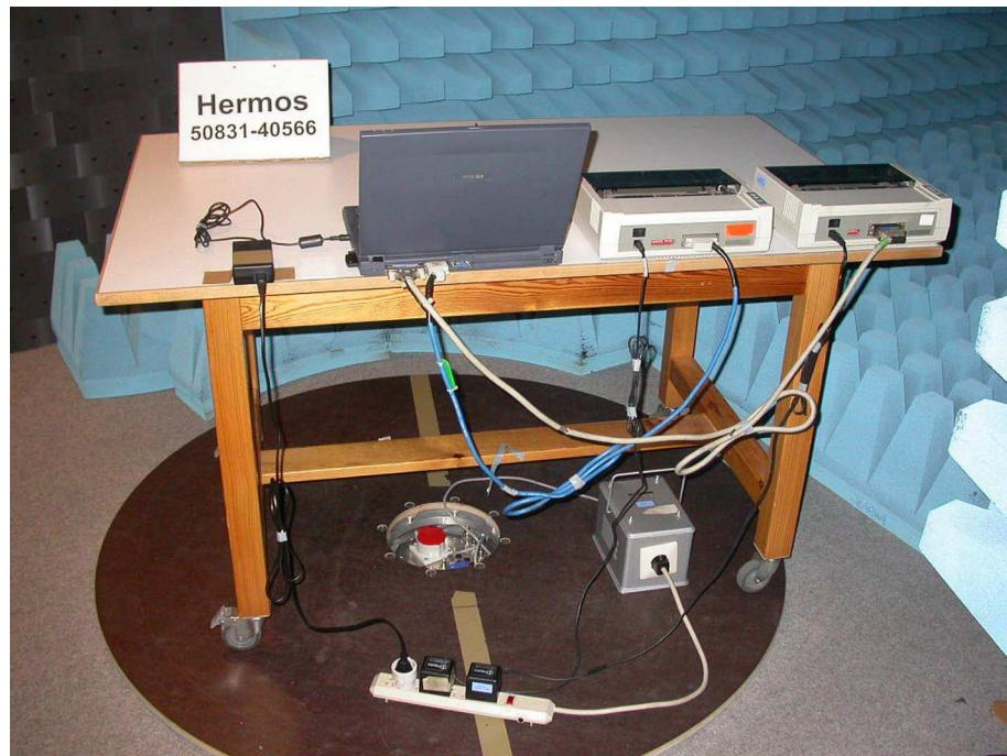
**Test setup for radiated emission test
