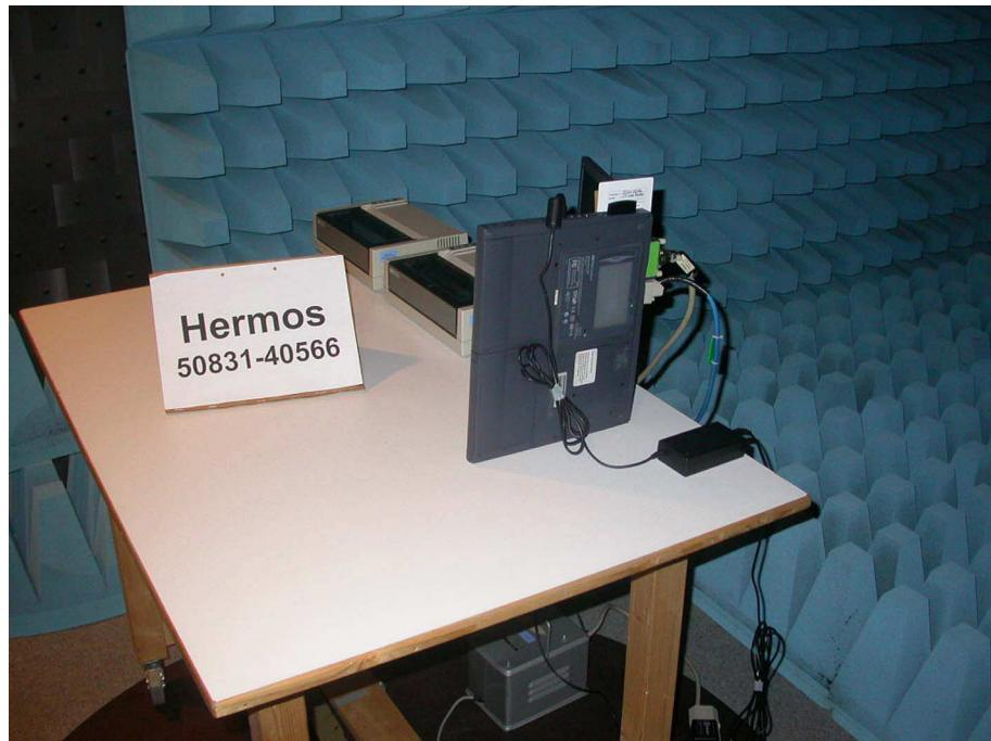
**Test setup for radiated emission test
