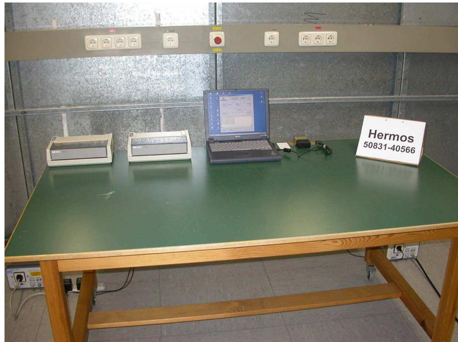
**Test setup for conducted AC powerline emission test - continued -**
