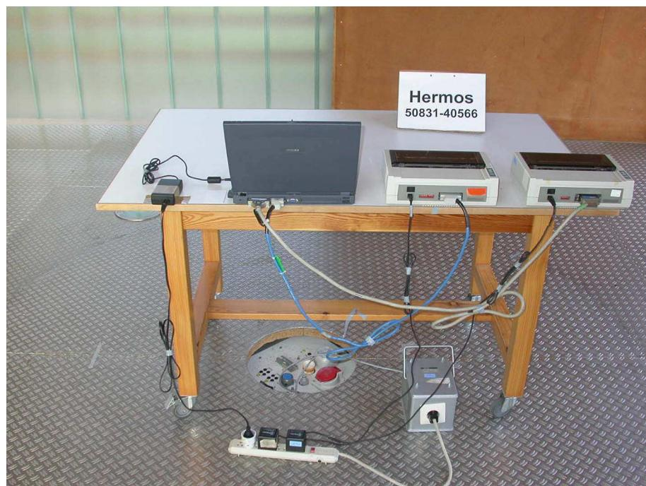
**Test setup for radiated emission test
