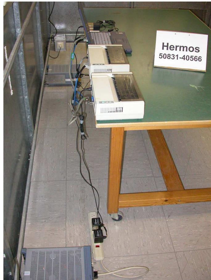
**Test setup for conducted AC powerline emission test - continued -**
