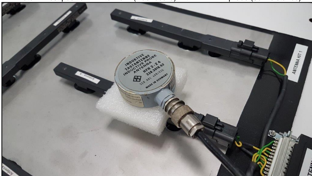
Photo 4: Test position - Antenna A (Dashboard) with HFH2-Z4 probe (3cm distance)
