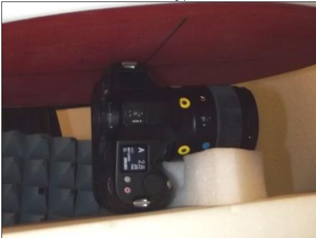
Photo 17: Measurement Position – Left Side with 0mm distance (MSL – ELI Phantom) with Multifunction Handgrip S attached
