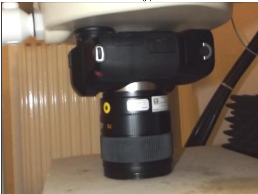
Photo 16: Measurement Position – Front with 0mm distance (HSL – SAM Phantom) with Multifunction Handgrip S attached
