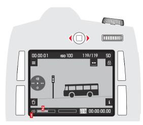
Turning the rear thumbwheel allows you to select other pictures. Turning to the left takes you to the pictures with lower numbers, turning to the right to the pictures with higher numbers. After reaching the highest and lowest
