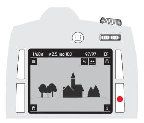
During both the unlimited review and the video payback, various additional displays and information can be called up in turn, in addition to the displays described above, by repeatedly pressing the button bottom right next to the monitor as in Live View mode:
