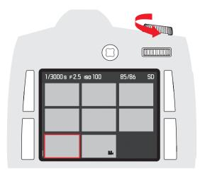
Turning the shutter speed setting dial to the left reduces possibly previously enlarged pictures, and turning beyond the review of the whole picture allows simultaneous viewing of 4 or 9 pictures.
