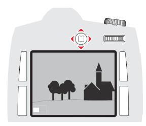
Press the Joystick in the desired direction - up, down, right or left
