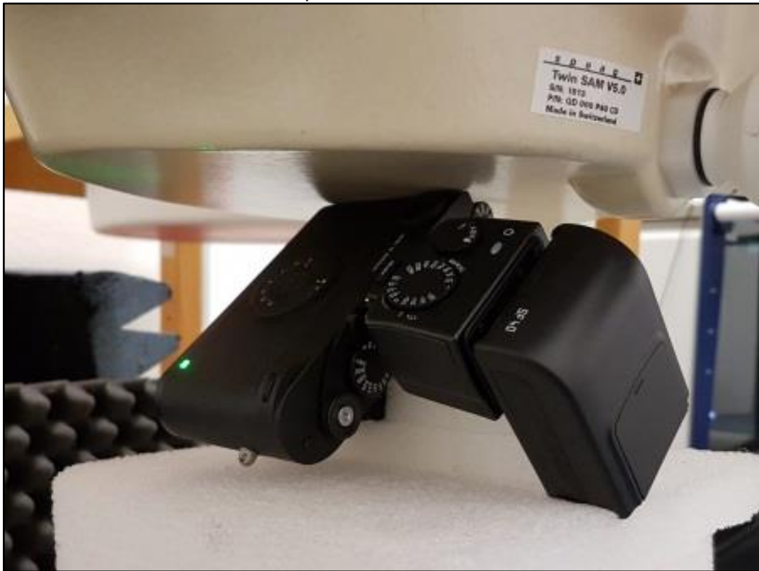
Photo 13: Test position rear 30° with Flash SF 40
