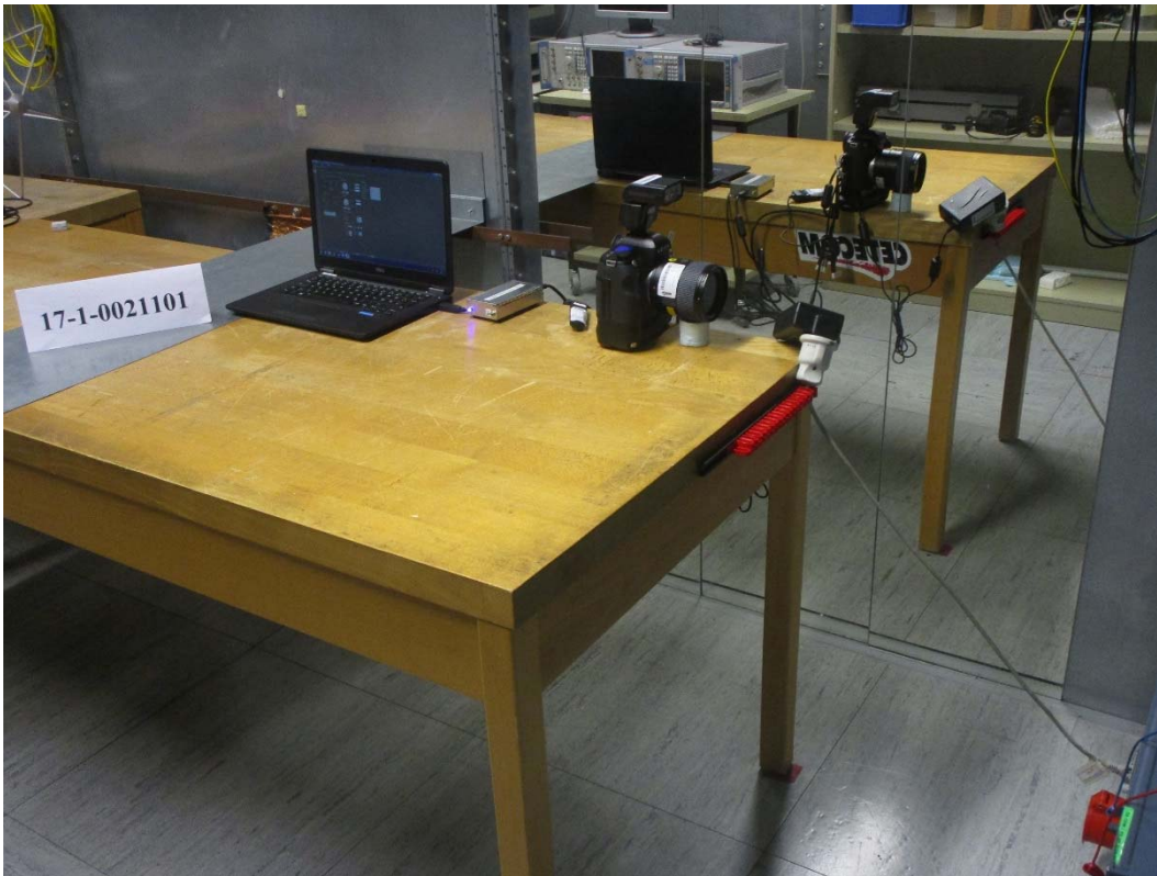
Photograph 1: Conducted measurements test set-up for AC-mains emission measurements
