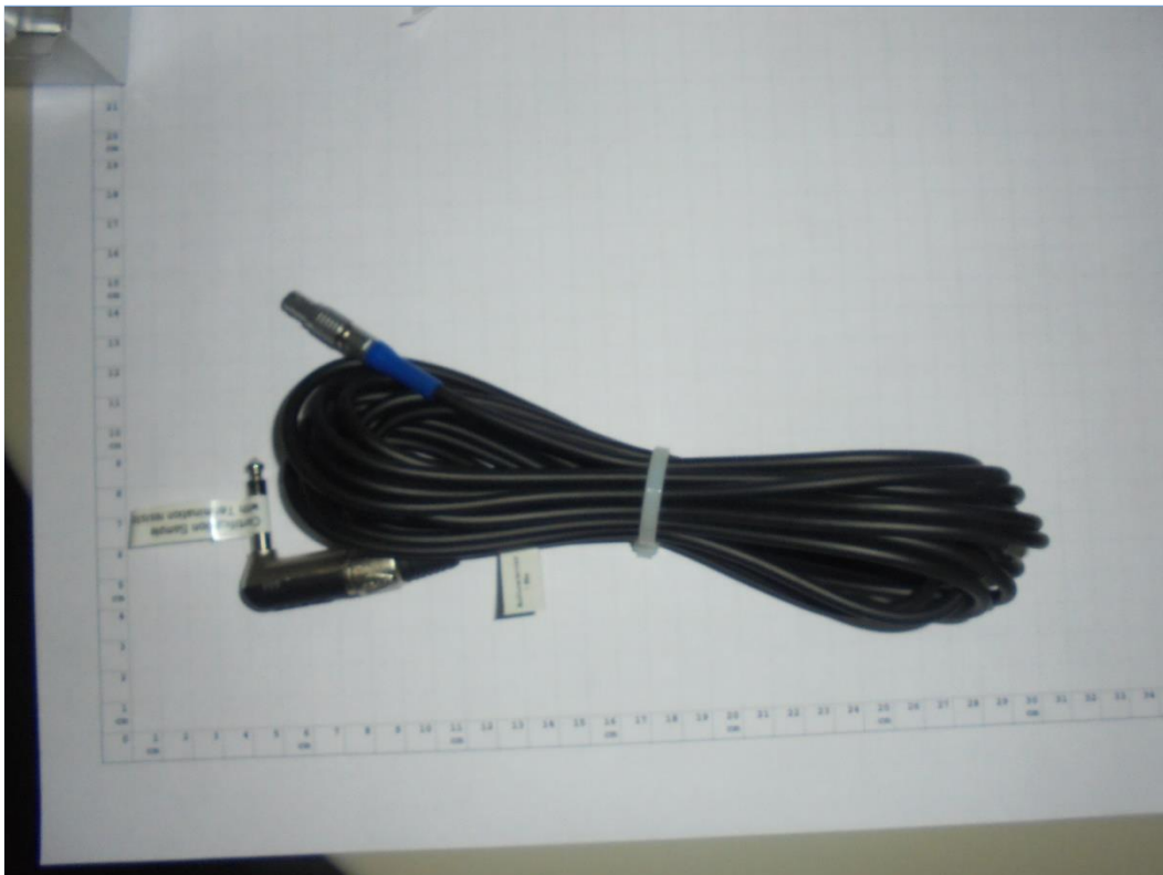
Photograph 8: Auxiliary equipment under test (AE 4), Flash Synchro cable S, Type: 16031
