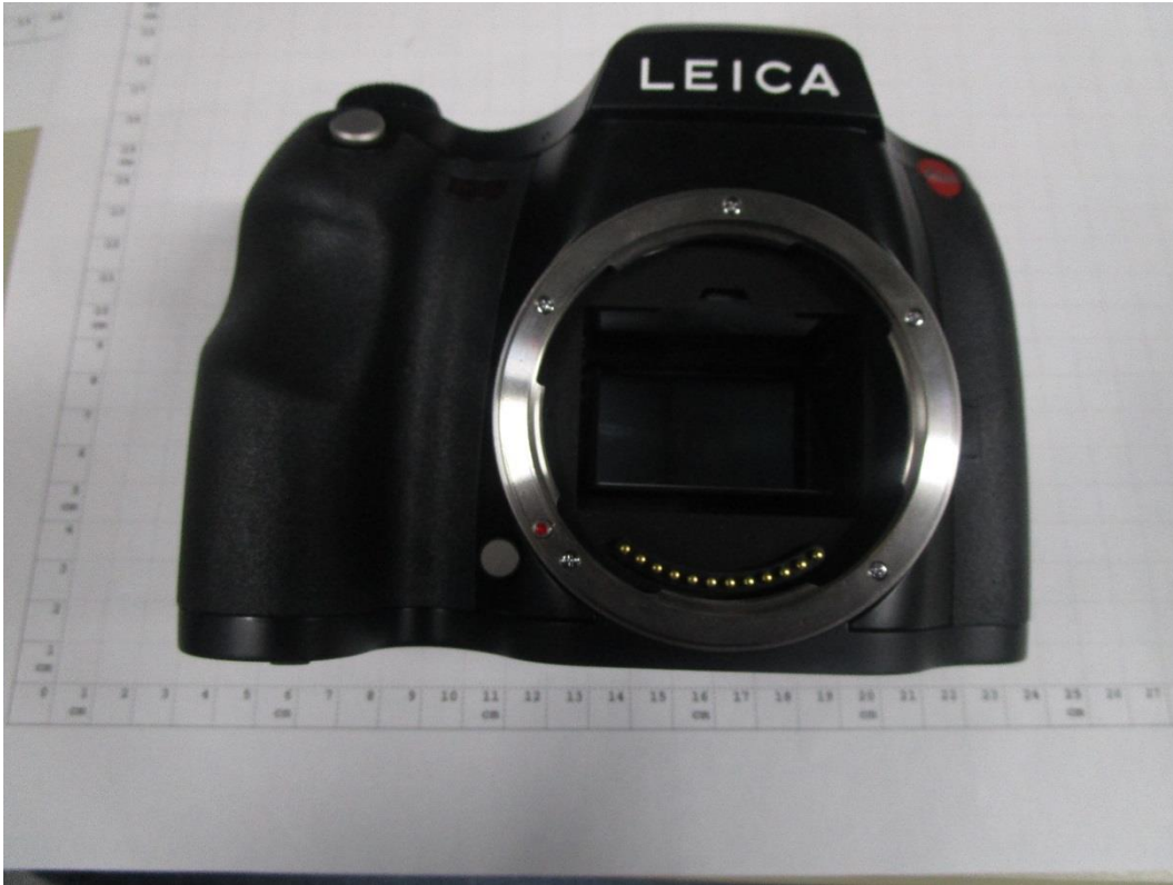
Photograph 1: Equipment under test (EUT A, front side) Leica Digital Camera S3, Type 6847
