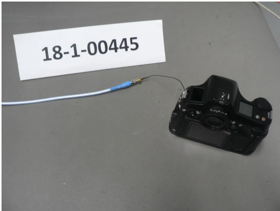
Photograph 8: Set-up for power measurements
