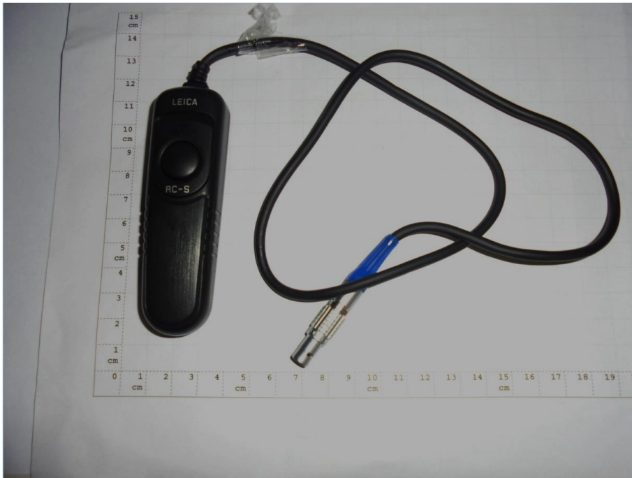
Photograph 13: Auxiliary equipment under test (AE 10), Remote control cable , Type: 16029
