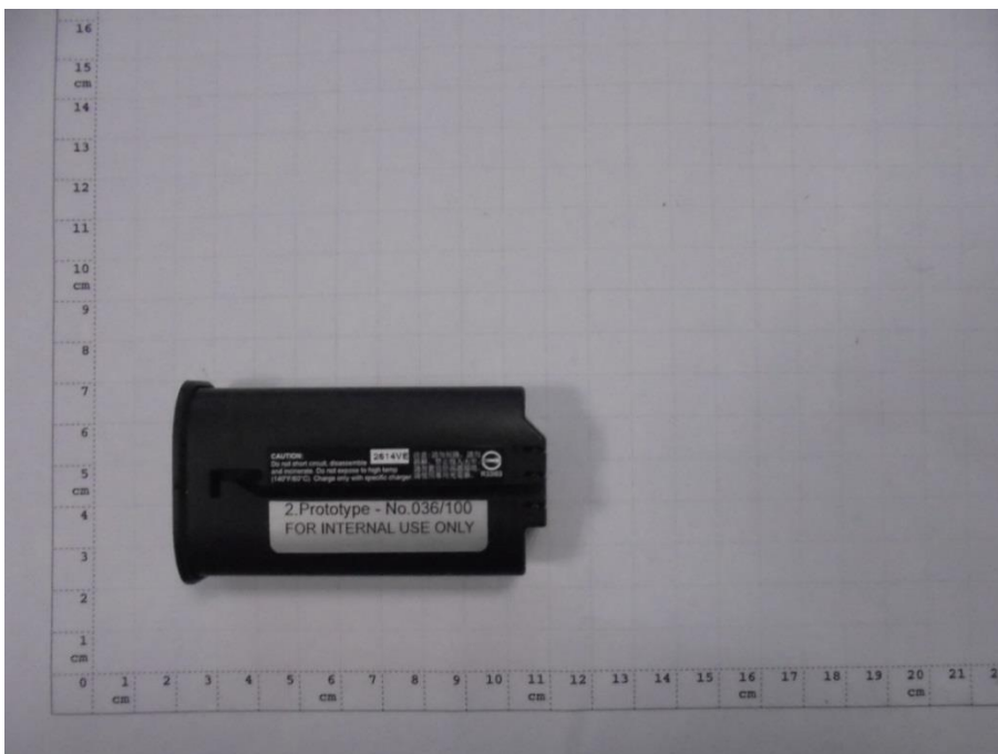
Photograph 6: Auxiliary equipment under test (AE 2), Li-ion Battery, Type: BP-PRO1, SN: 1417VB
