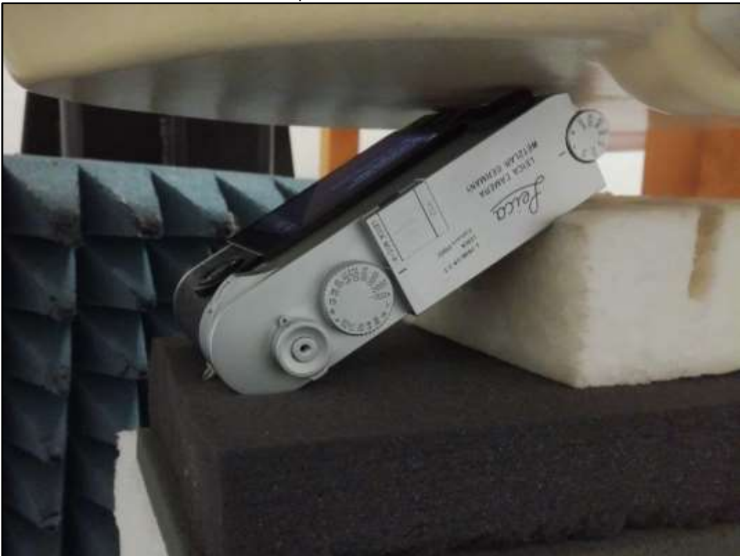
Photo 10: Test position rear 30° with metal cover
