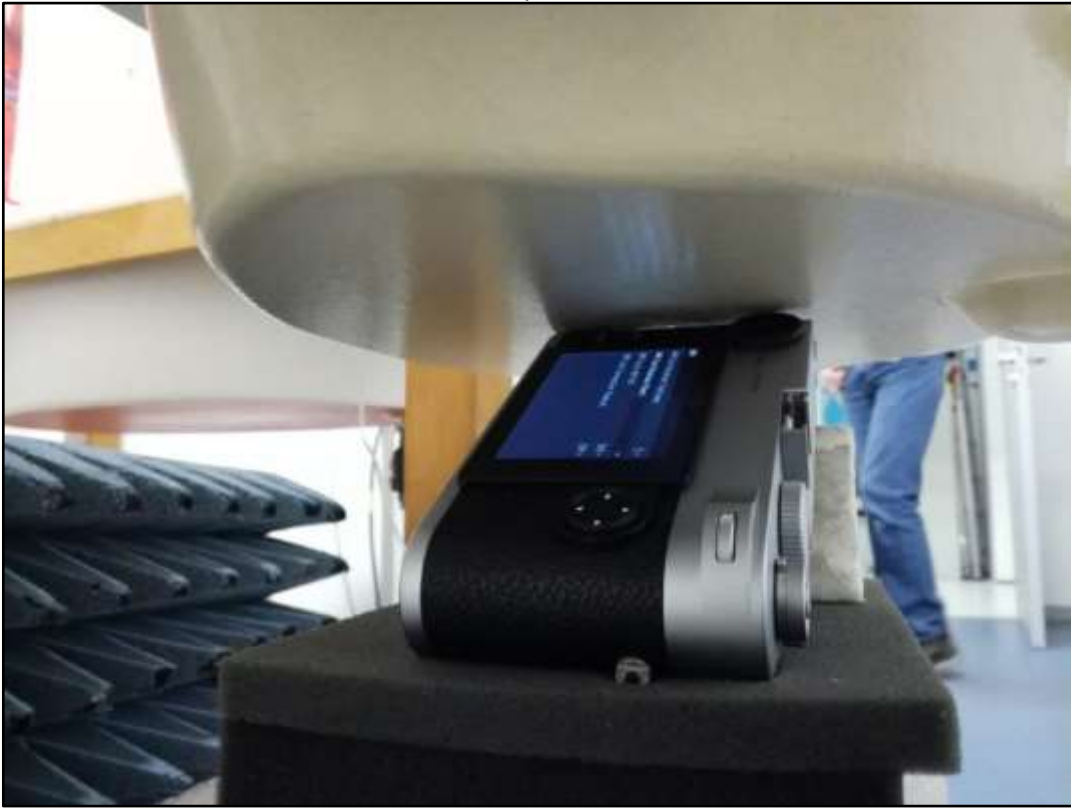
Photo 10: Test position rear 30° with metal cover
