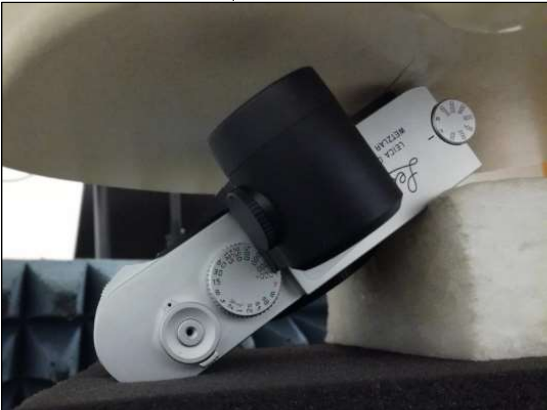
Photo 14: Test position rear 30° with Visoflex
