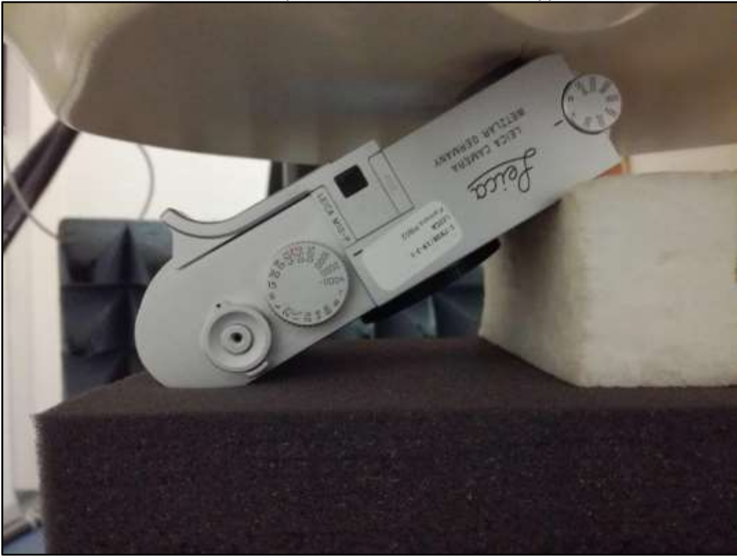
Photo 12: Test position rear 30° with handgrip
