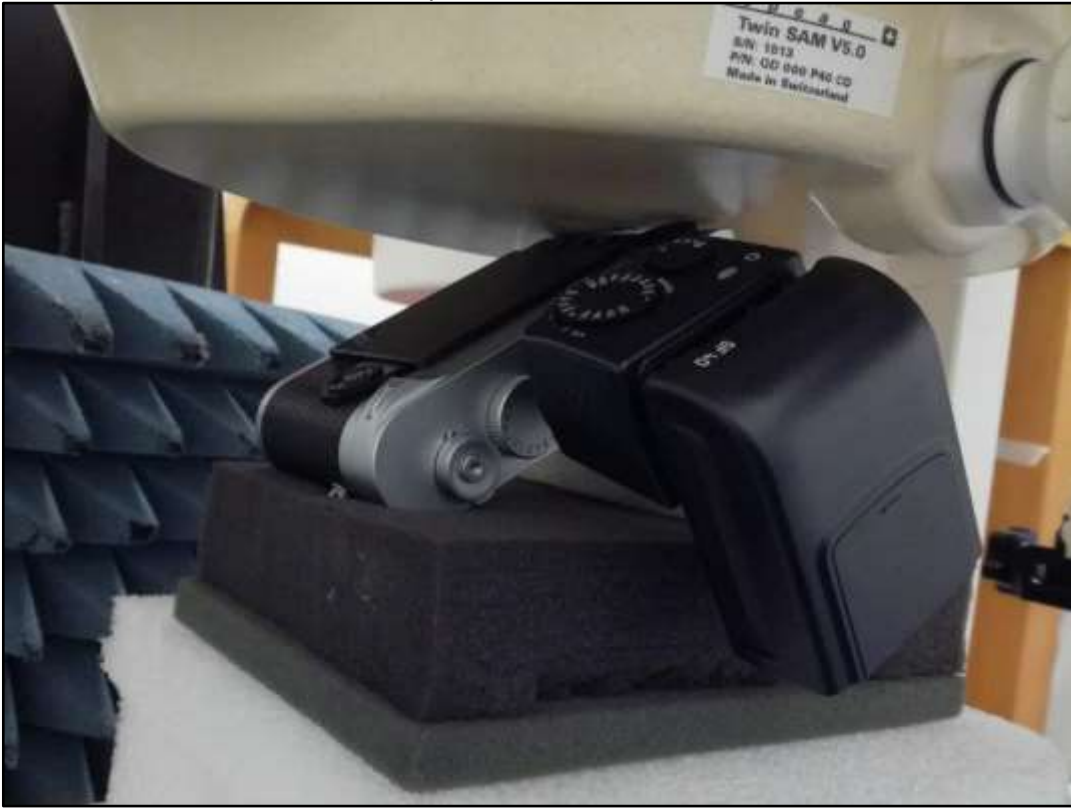
Photo 14: Test position rear 30° with Visoflex
