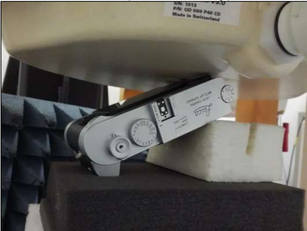
Photo 12: Test position rear 30° with handgrip
