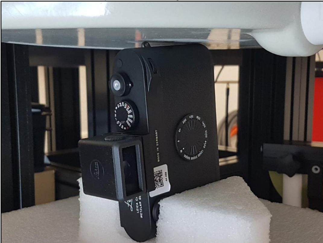
Photo 18: Test position limb worn right side with 0 mm distance
