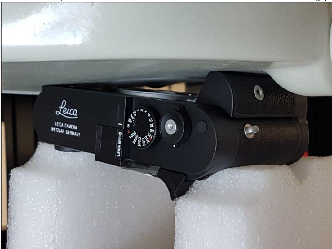
Photo 22: Test position limb worn back side with 0 mm distance with thumb and handgrip
