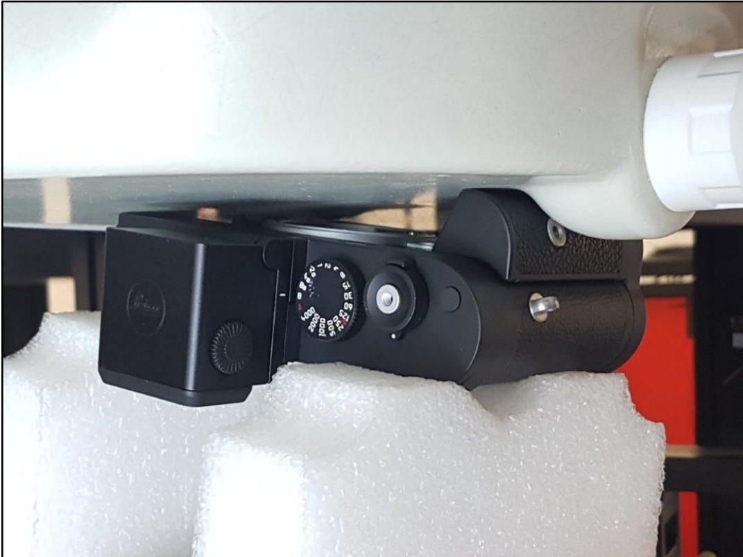
Photo 22: Test position limb worn back side with 0 mm distance with thumb and handgrip
