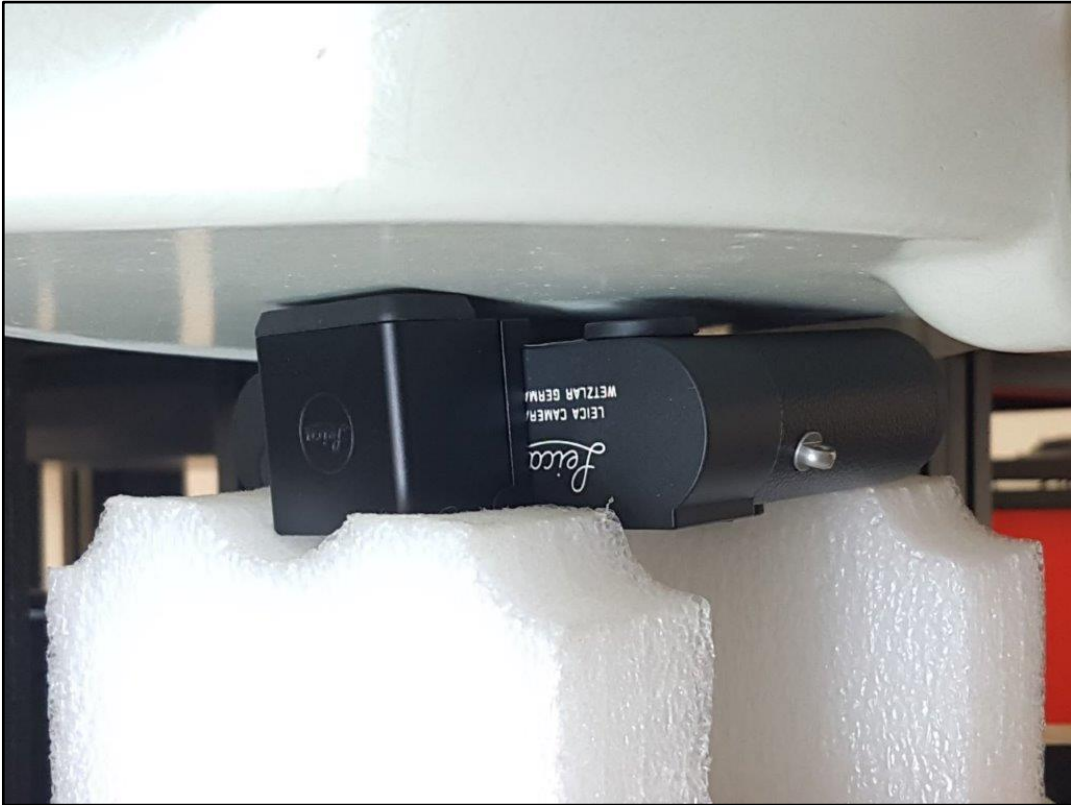
Photo 16: Test position body and head worn top side with 0 mm distance
