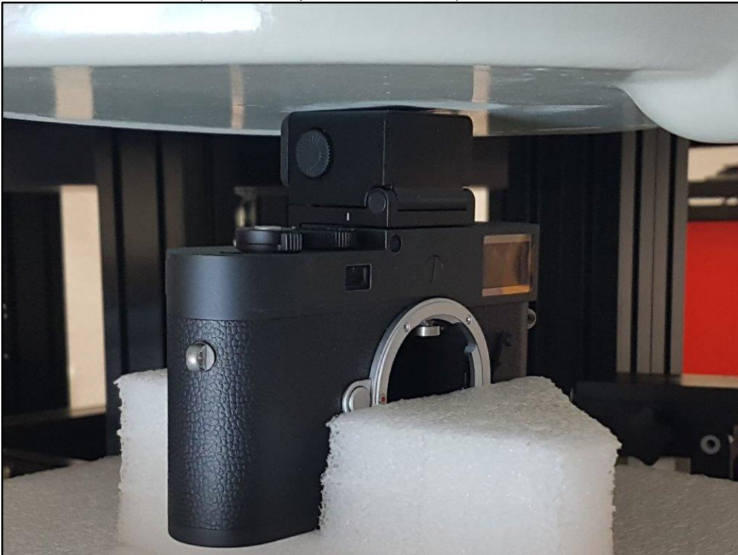
Photo 16: Test position body and head worn top side with 0 mm distance
