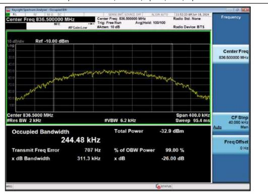
Occupied Bandwidth / Cellular / Uplink / GSM / Input
