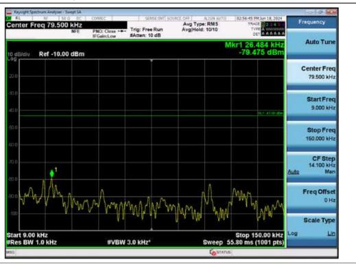
Conducted Spurious Emissions / Broadband PCS / Downlink / 9 kHz ~ 150 kHz
