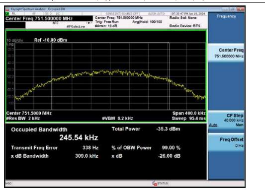
Occupied Bandwidth / Upper 700 MHz / Downlink / GSM / Input
