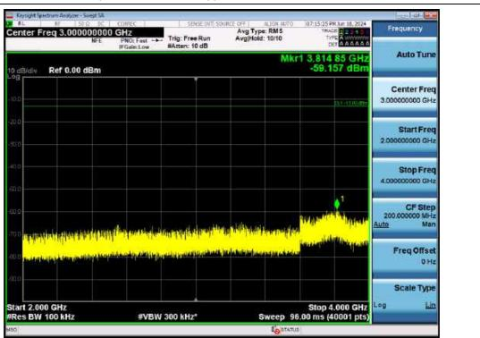
Conducted Spurious Emissions / Upper 700 MHz / Downlink / 2 GHz ~ 4 GHz
