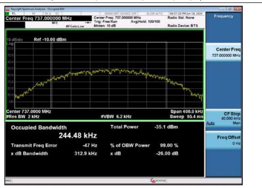
Occupied Bandwidth / Lower 700 MHz / Downlink / GSM / Input
