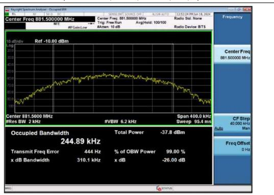
Occupied Bandwidth / Cellular / Downlink / GSM / Input
