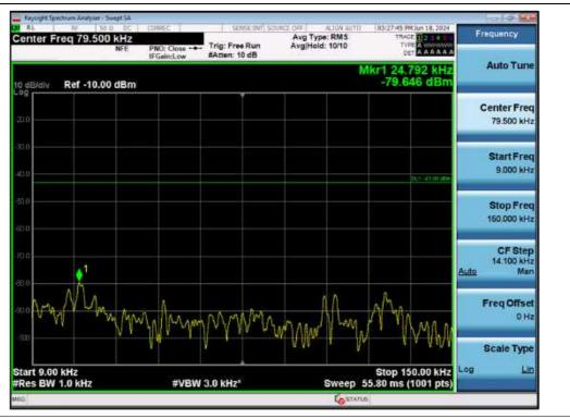
Conducted Spurious Emissions / AWS-1 / Downlink / 9 kHz ~ 150 kHz
