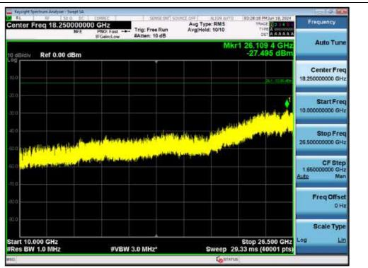
Conducted Spurious Emissions / AWS-1 / Downlink / 10 GHz ~ 26.5 GHz
