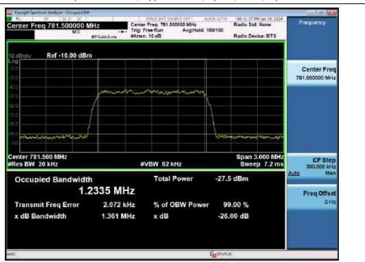
Occupied Bandwidth / Upper 700 MHz / Uplink / CDMA/ Input
