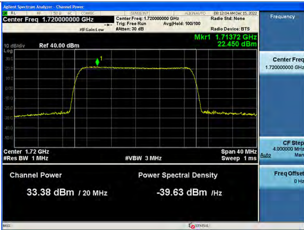
3 dB above the AGC threshold PSD / AWS / Uplink / 5G NR 20 MHz
