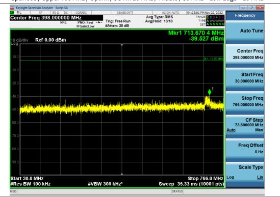
Spurious / Upper 700 MHz / Uplink / 5G NR 10 MHz / Middle / 30 MHz ~ Low Edge - 10 MHz
