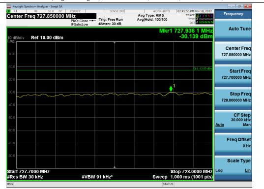
Out-of-band (single test signal) / Lower 700 MHz / Downlink / 5G NR 10 MHz / Lower
