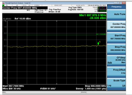
Out-of-band (single test signal) / Lower 700 MHz / Uplink / 5G NR 10 MHz / Lower
