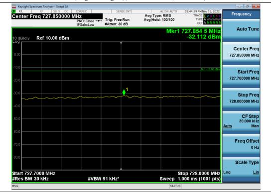
+3 dB above Out-of-band (single test signal) / Lower 700 MHz / Downlink / 5G NR 10 MHz / Lower
