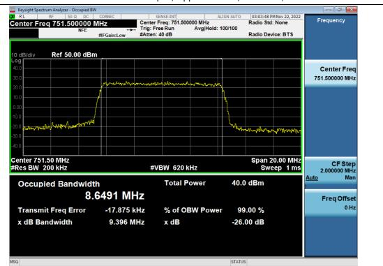
3 dB above the AGC threshold output / Upper 700 MHz / Downlink / 5G NR 10 MHz
