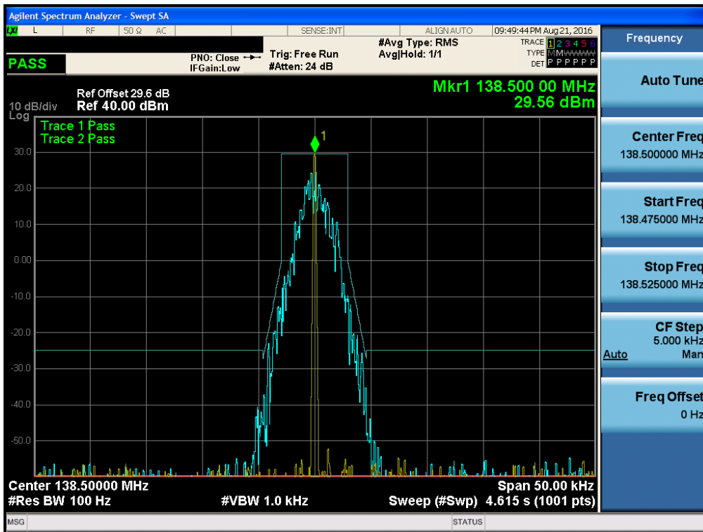
[138.5 MHz Downlink Emission Mask E]
