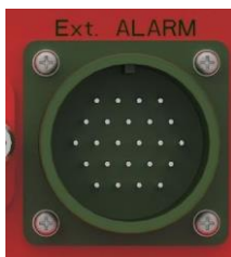
Figure 3-3 External Alarm Port
