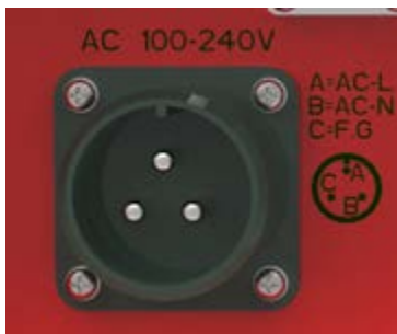
Figure 2-3 AC Input Port
