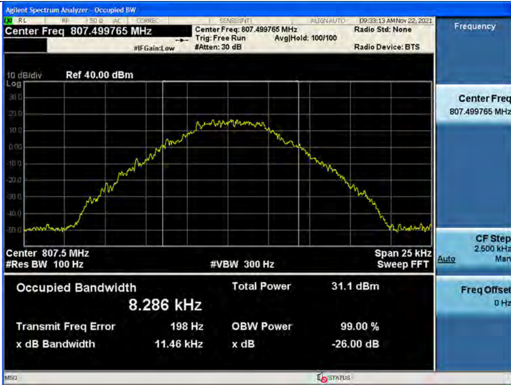
Output / NPSPAC / Uplink / P25 Phase 1
