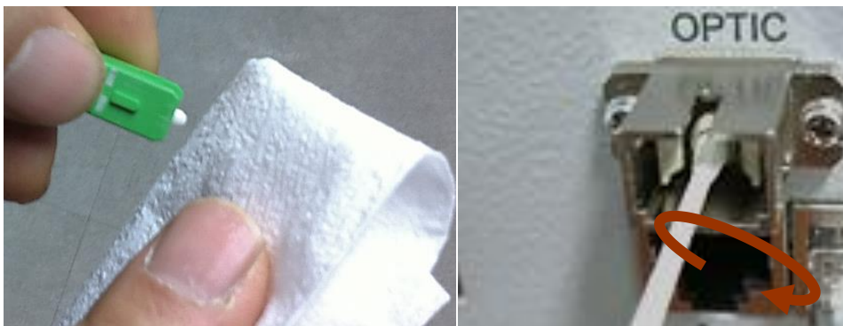
Figure 3-7 Optic Connector Cleaning (left) and Optic Port Cleaning (right)
