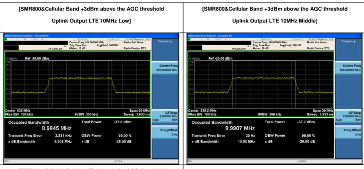
[SMR800&Cellular Band +3dBm above the AGC threshold
