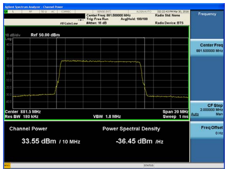
SMR 800&Cellular Band_ AGC threshold Downlink (869 MHz~894 MHz) Middle]
