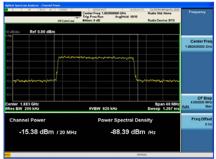
[PCS 1900 +3dB above the AGC threshold Uplink LTE 20MHz Mid]
