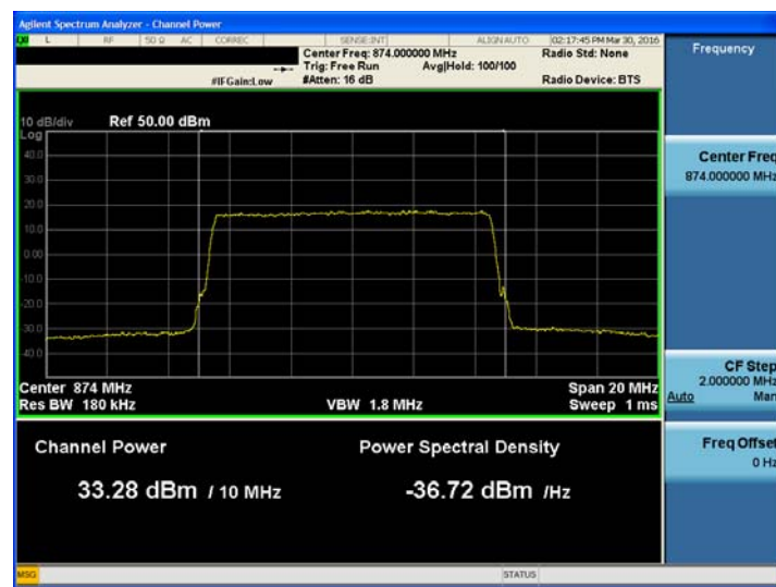
SMR 800&Cellular Band_ AGC threshold Downlink (869 MHz~894 MHz) High]
