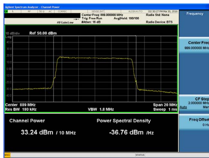
SMR 800&Cellular Band_ AGC threshold Downlink (869 MHz~894 MHz) High]
