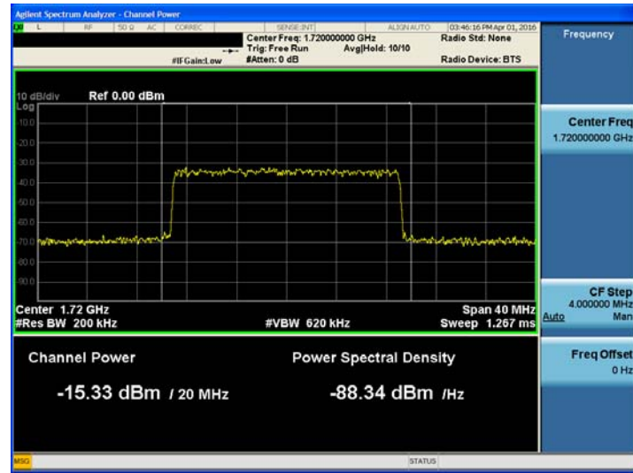
[AWS 2100 AGC threshold Uplink LTE 20MHz High]
