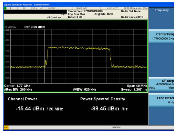
[AWS 2100 AGC threshold Uplink LTE 20MHz High]
