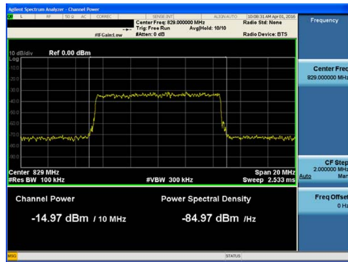
[SMR 800, Cellular +3dB above the threshold Uplink LTE 10 MHz High]
