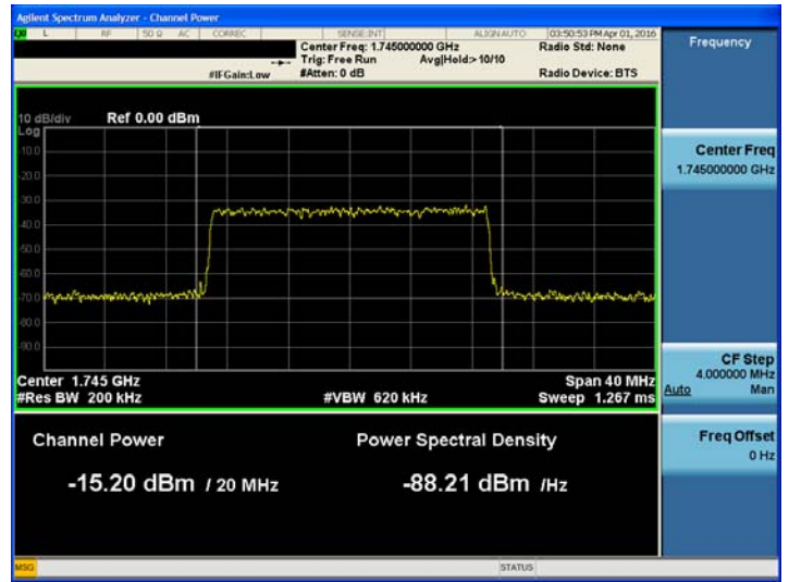
[AWS 2100 AGC threshold Uplink LTE 20MHz Mid]
