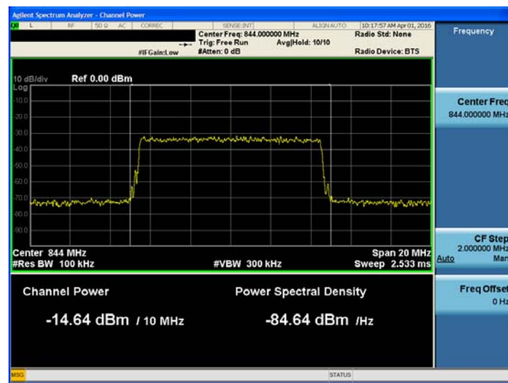
[SMR 800, Cellular +3dB above the threshold Uplink LTE 10 MHz High]
