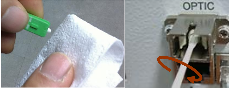
Figure 6-5 Optic Connector Cleaning (left) and Optic Port Cleaning (right)
