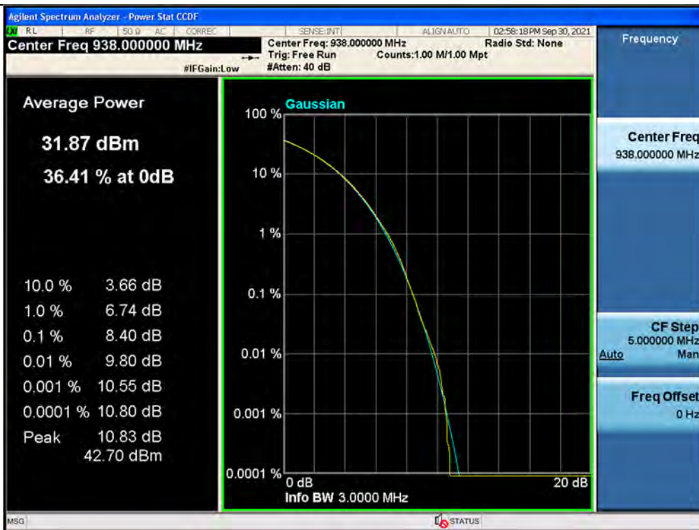
PAPR / 900 MHz Broadband / Downlink / LTE 3 MHz
