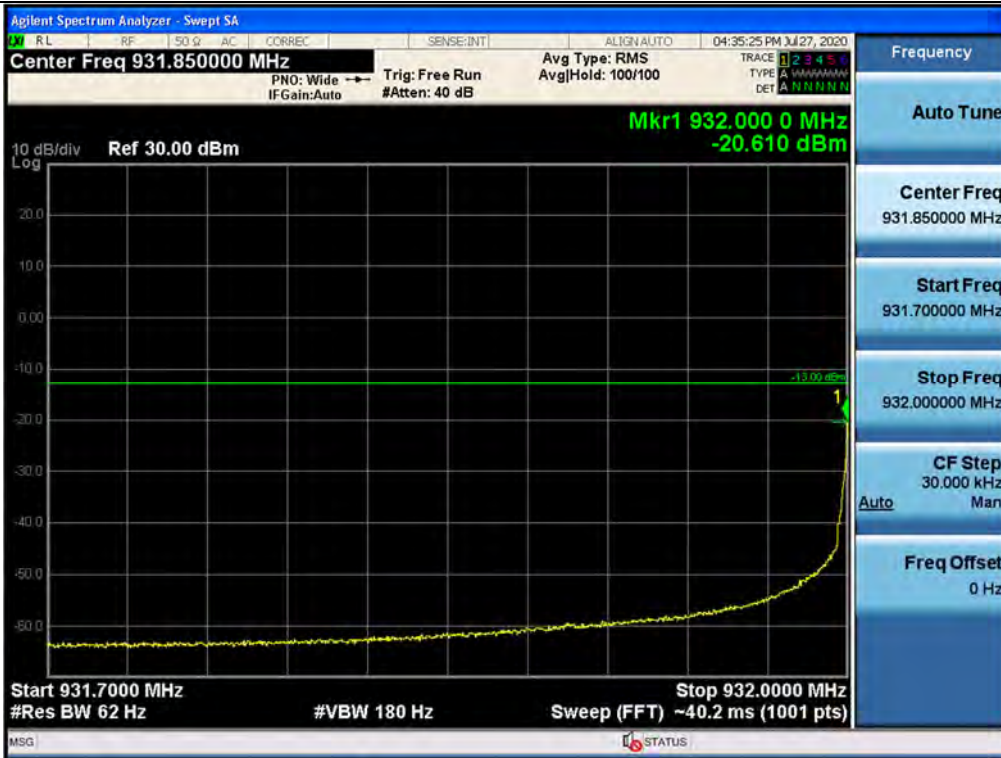
+3 dB above Out-of-band (single test signals) / 932 ~ 935 MHz / Downlink / P25 Phase 2 / Lower
