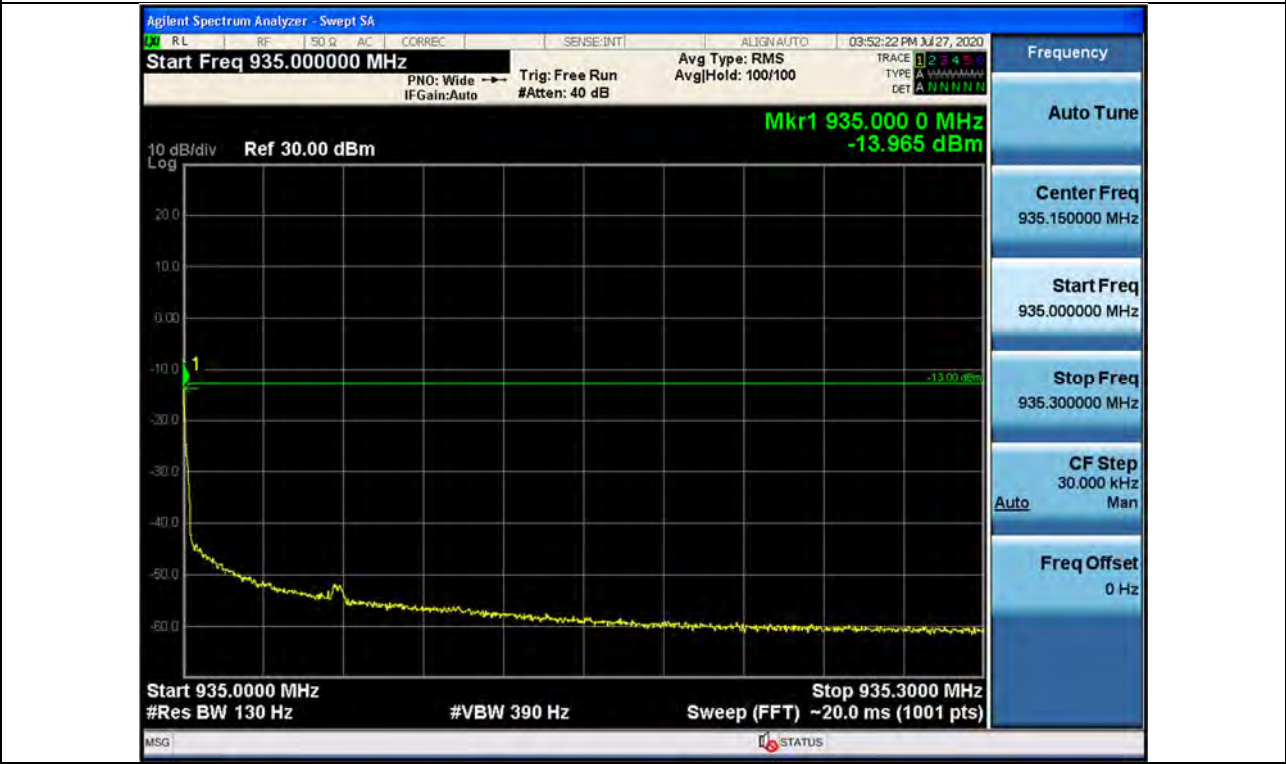
Out-of-band (single test signals) / 932 ~ 935 MHz / Downlink / P25 Phase 1 / Upper
