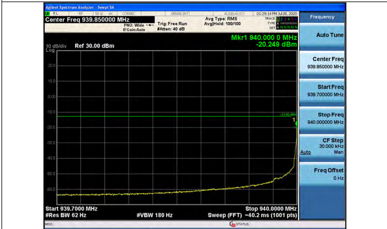
+3 dB above Out-of-band (single test signals) / 940 ~ 941 MHz / Downlink / P25 Phase 2 / Lower
