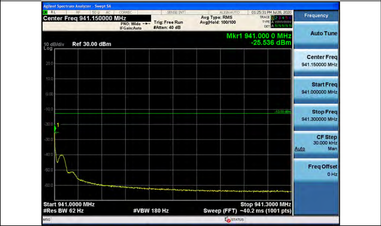
Out-of-band (two adjacent test signals) / 940 ~ 941 MHz / Downlink / P25 Phase 2 / Upper
