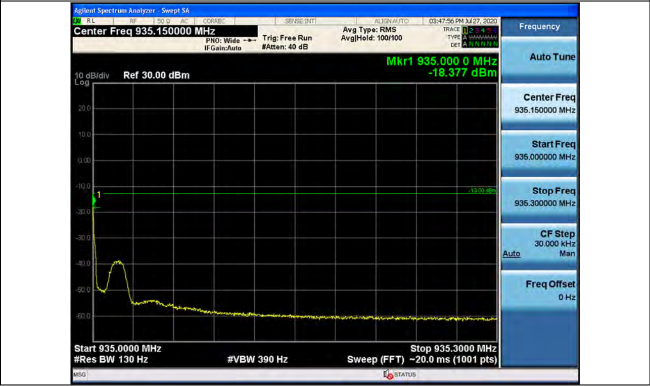
+3 dB above Out-of-band (two adjacent test signals) / 932 ~ 935 MHz / Downlink / P25 Phase 1 / Upper
