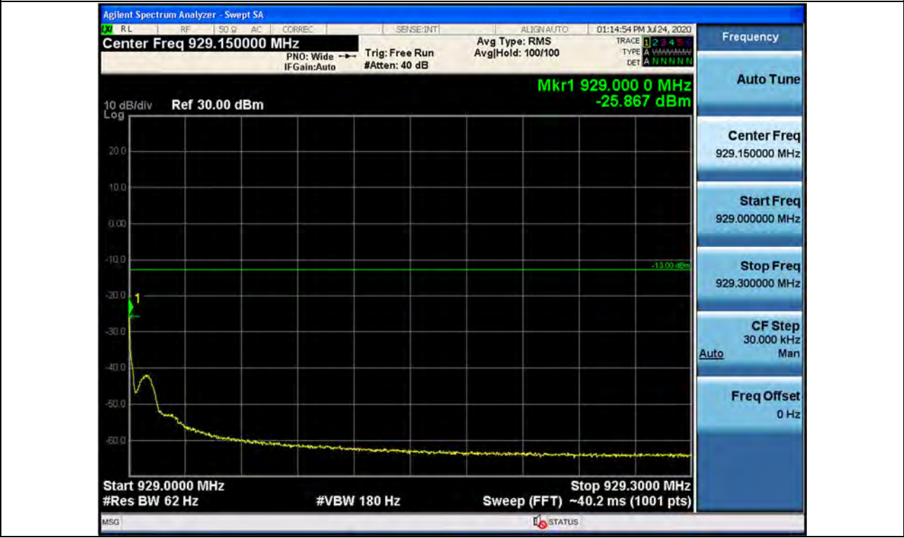
+3 dB above Out-of-band (two adjacent test signals) / 928 ~ 929 MHz / Downlink / P25 Phase 2 / Upper
