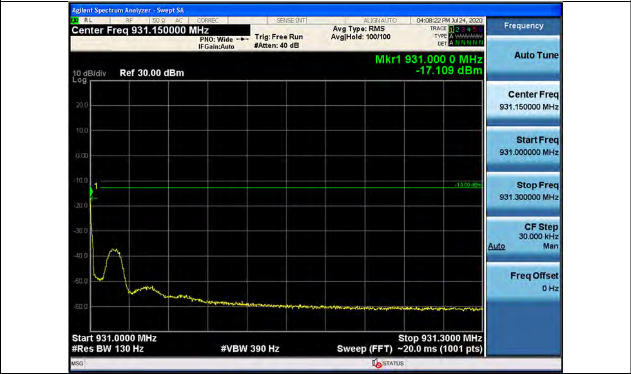
Out-of-band (two adjacent test signals) / 930 ~ 931 MHz / Downlink / P25 Phase 1 / Upper
