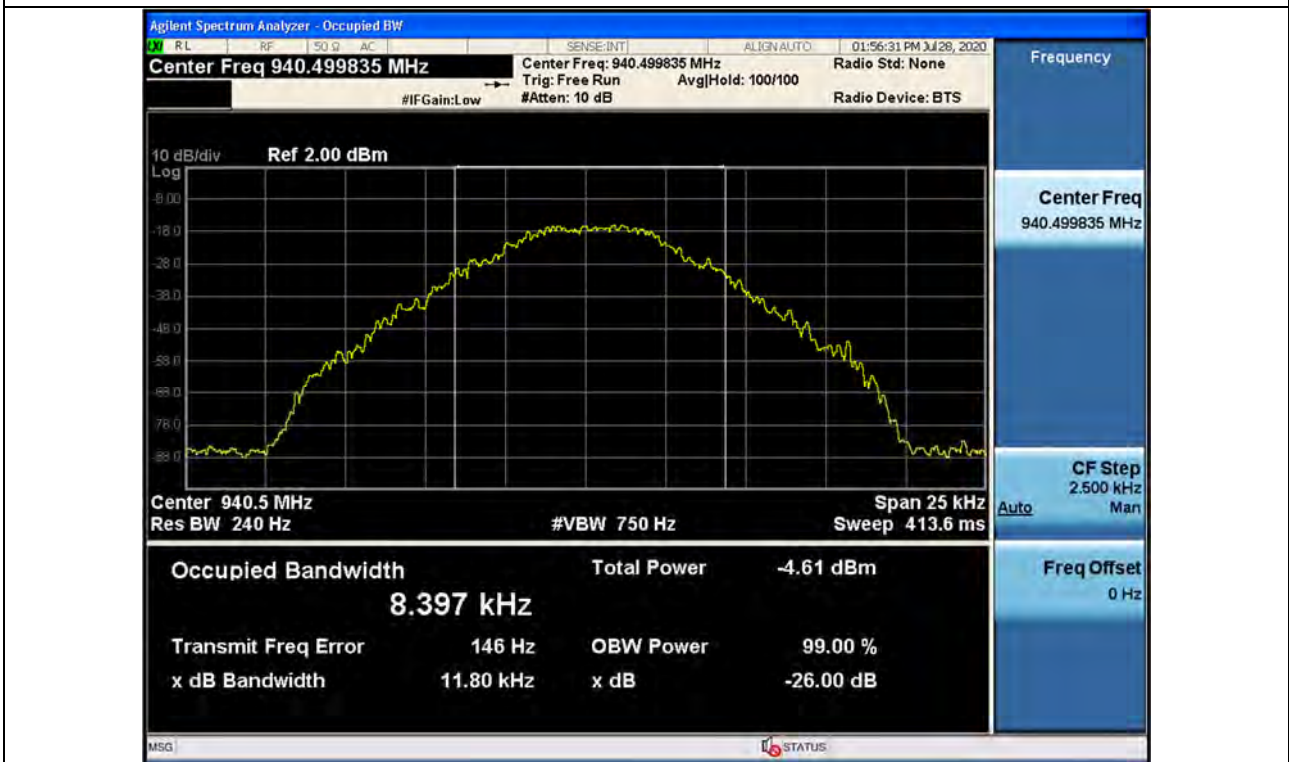
3 dB above the AGC threshold Input / 940 ~ 941 MHz / Downlink / P25 Phase 1
