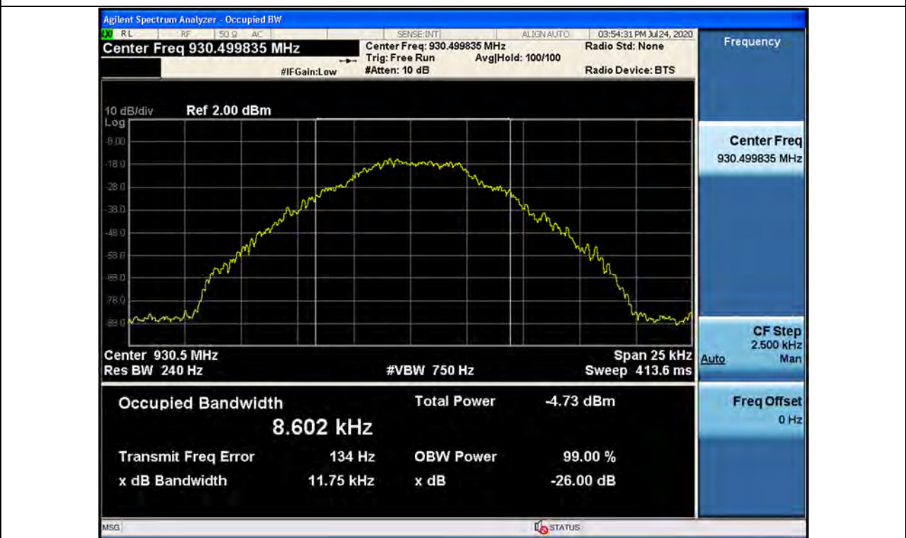
3 dB above the AGC threshold Input / 930 ~ 931 MHz / Downlink / P25 Phase 1
