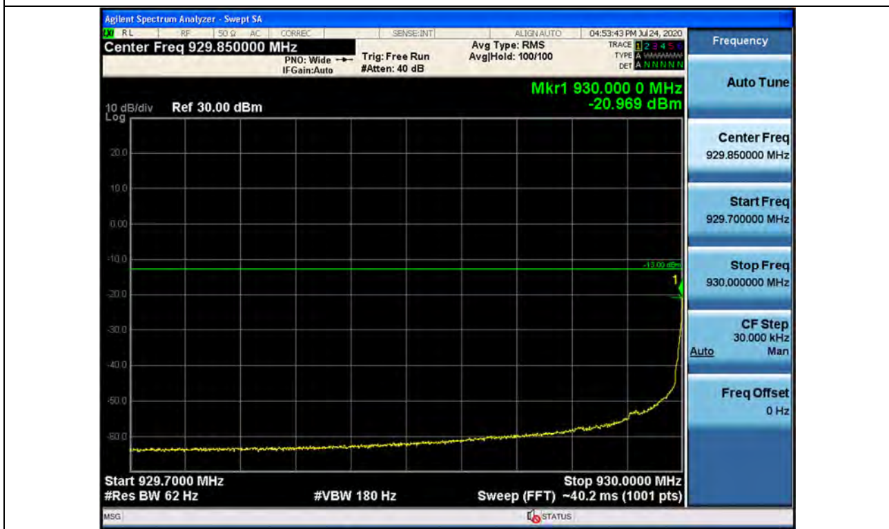
Out-of-band (single test signals) / 930 ~ 931 MHz / Downlink / P25 Phase 2 / Lower
