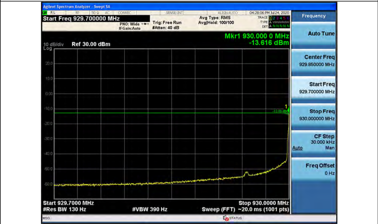
Out-of-band (single test signals) / 930 ~ 931 MHz / Downlink / P25 Phase 1 / Lower
