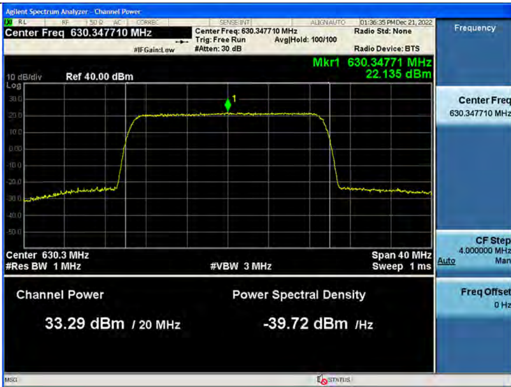
3 dB above the AGC threshold PSD / 600 MHz Service / Downlink / 5G NR 20 MHz
