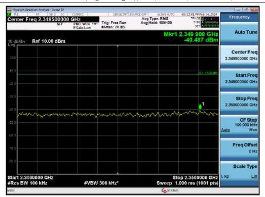
+3 dB above Out-of-band (single test signal) / WCS / Downlink / 5G NR 10 MHz / Lower
