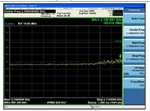
+3 dB above Out-of-band (single test signal) / AWS / Downlink / LTE 20 MHz / Lower
