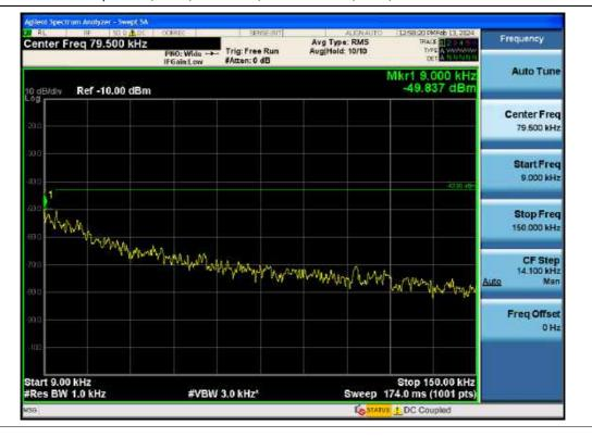
Spurious / AWS / Downlink / 5G NR 60 MHz / Low / 9 kHz ~ 150 kHz
