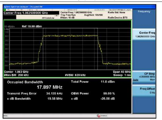
3 dB above the AGC threshold Input / PCS / Downlink / LTE 20 MHz
