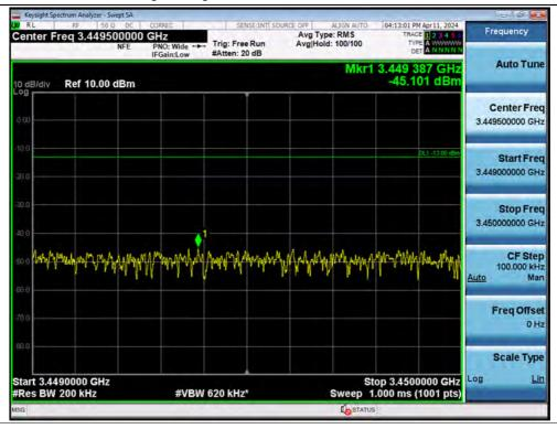
+3 dB above Out-of-band (single test signal) / 3.45 GHz Service / Downlink / Ant. 2 / 5G NR 100 MHz / Upper
