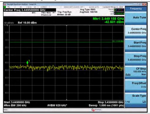
+3 dB above Out-of-band (single test signal) / 3.45 GHz Service / Downlink / Ant. 1 / 5G NR 100 MHz / Upper
