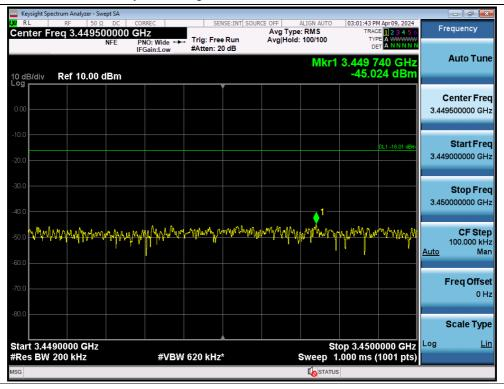
+3 dB above Out-of-band (two adjacent test signals) / 3.45 GHz Service / Downlink / Ant. 2 / 5G NR 100 MHz / Upper
