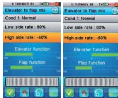
升降舵摇杆打到最下边 The elevator to the topside (Pic 22.4) 升降舵摇杆打到最上边 The elevator to the bottom (Pic 22.5)
